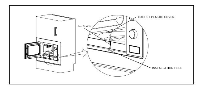
• Open the door; fix the oven to the cabinet with SCREW B at the INSTALLATION HOLE of TRIM KIT. Then fix the TRIM-KIT PLASTIC COVER to the INSTALLATION HOLE.
